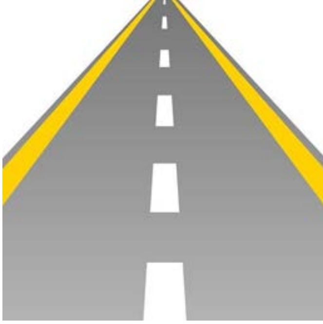
Broken White Line
